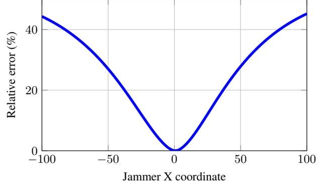
**Fig. 1.** Relative error between the approximated function  $\mathbb{E}\{C_t(S_x, S_y)\}$  and the average of 100 realizations  $\mathbb{E}\{C_t(S_x, S_y)\}$ . Communicator is fixed in  $(x_c, y_c) = (2, 1)$  and the jammer is moved along main diagonal ( $x_j = y_j$ ). The error is smaller when the hypotheses are satisfied and both UAVs are far from the edges ( $|x_c|, |y_c| \ll D$  and  $|x_j|, |y_j| \ll D$ ).
